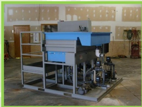
50 GPM "Electro Coagulation" Unit
