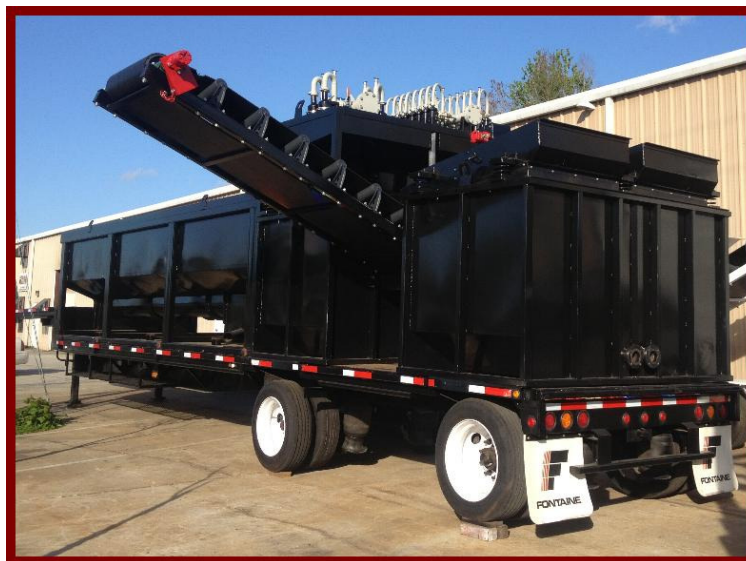
Oilfield Wellhead Mobile Remediation Service Unit Processes 60 Tons Per Hour
