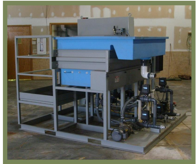
Electro Coagulation Unit 50 Gallons Per Minute
