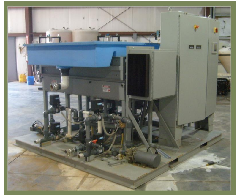
Electro Coagulation Unit 50 Gallons Per Minute
